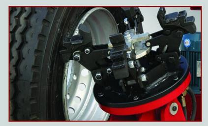
Unique clamps to fit the aluminum wheels with jaw protectors to keep the aluminum rims from damaging.
