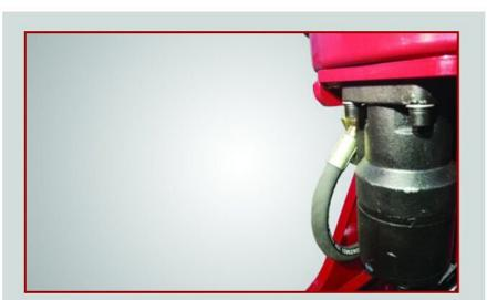
Hydraulic motor transmission with large diameter oil tube obviously improves working efficiency.
