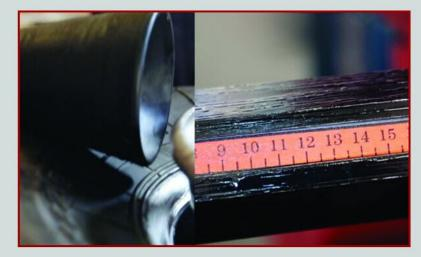
Pusher block can be adjusted freely while working, and with the gauge help, It can be fixed according to wheel rim position.
