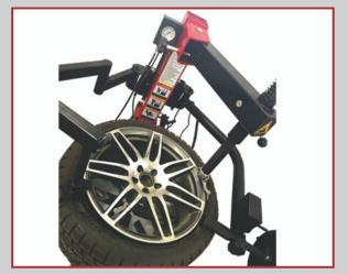
Three points press the tires together with the helper, making it easier to change the tire and improves the working rate.
