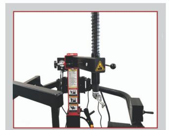
Uses one cylinder to support both the right and left assist arms at the same time. Easy to operate and improves the working rate.
