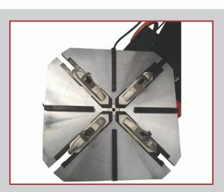
Double-wear resist scribing's makes wheel clamps move more fluently. The limited block avoids scratching wheels and can fix the position for tires on the wheel clamps automatically.
