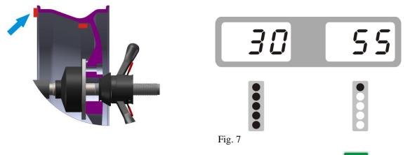
4.2.7. After finishing mounting the counterweights, put down the guard or press **START**, to perform balancing spin again, if comes out 00 00, means balancing succeed. (Fig.8)
