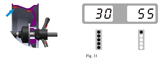
After finishing mounting the counterweights, put down the guard and press **START**, to perform balancing spin again, if comes out 00 00, means balancing succeed. (Fig.12)
