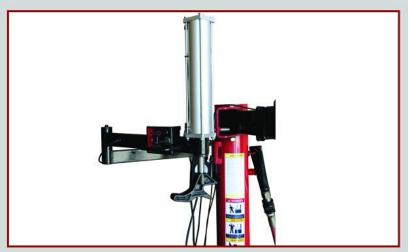
Swing arm fixed on rod will be safe and avoid cylinder explosion.
